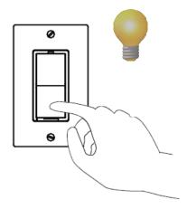
3) Press the pushbutton on the HAI UPB<sup>™</sup> 6-Button Room Controller five (5) times quickly.
